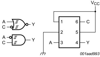
**Fig 8.** 2-input AND gate with input A inverted or
