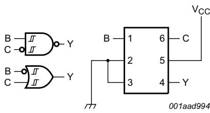
**Fig 9.** 2-input OR gate with input B inverted or
