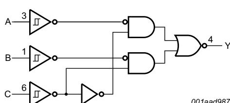
**Fig 1. Logic diagram**
