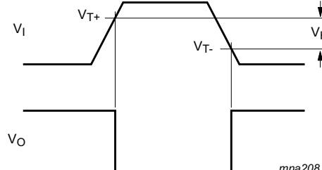
VT<sub>+</sub> and VT<sub>-</sub> limits at 70 % and 20 %.Fig 16. Definition of VT<sub>+</sub>, VT<sub>-</sub> and VH
