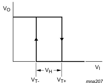
Fig 15. Transfer characteristic
