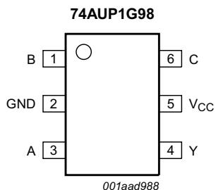
Fig 2. Pin configuration SOT363
