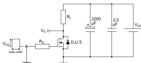
**Figure 14: Test circuit for gate charge behavior**
