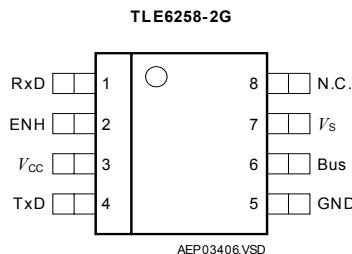
**Figure 1** Pin Configuration (top view)
