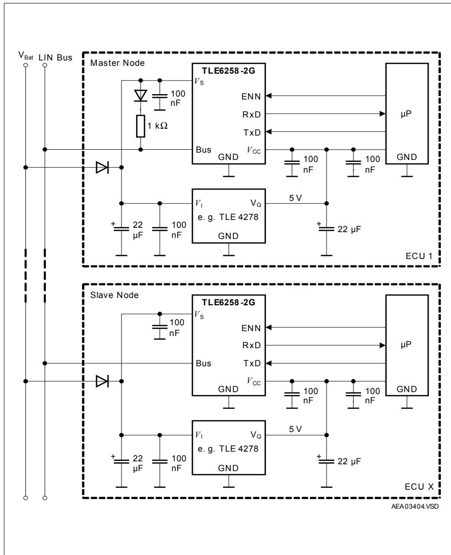
Figure 6 Application Circuit
