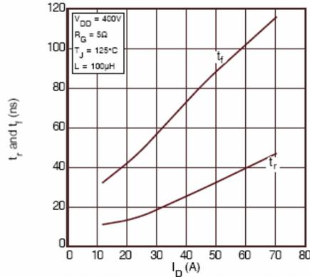
FIGURE 15, RISE AND FALL TIMES vs CURRENT
