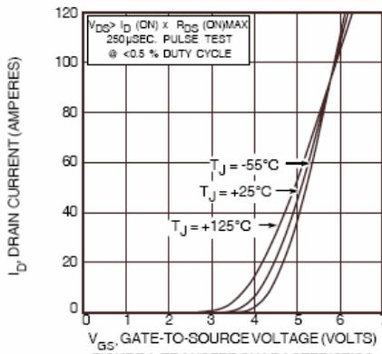
FIGURE 4, TRANSFER CHARACTERISTICS
