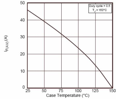
Figure 7. Maximum Average Forward Current vs. Case Temperature
