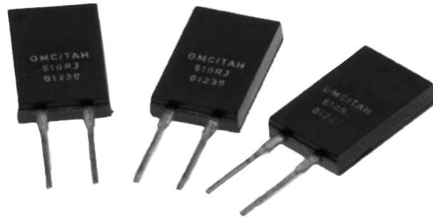
The TAH20 is a completely encapsulated thick film resistor in the T0220 package outline. Rated for 20 watts @ 25°C case temperature, these resistors are electrically isolated, and molded in a high temperature case.
