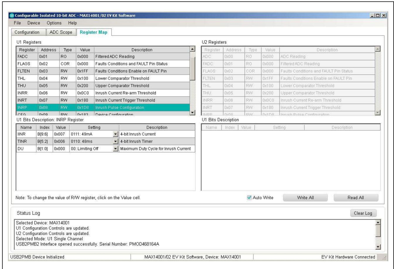
Figure 5. EV Kit Software (Register Map Tab)
