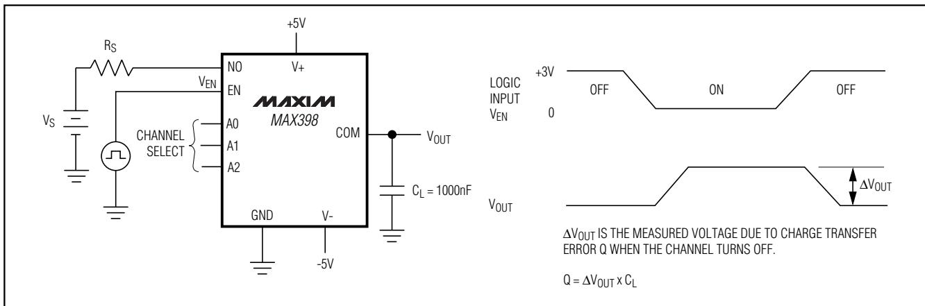
Figure 5. Charge Injection
