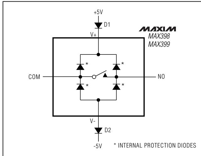
Figure 1. Overvoltage Protection Using External Blocking Diodes
