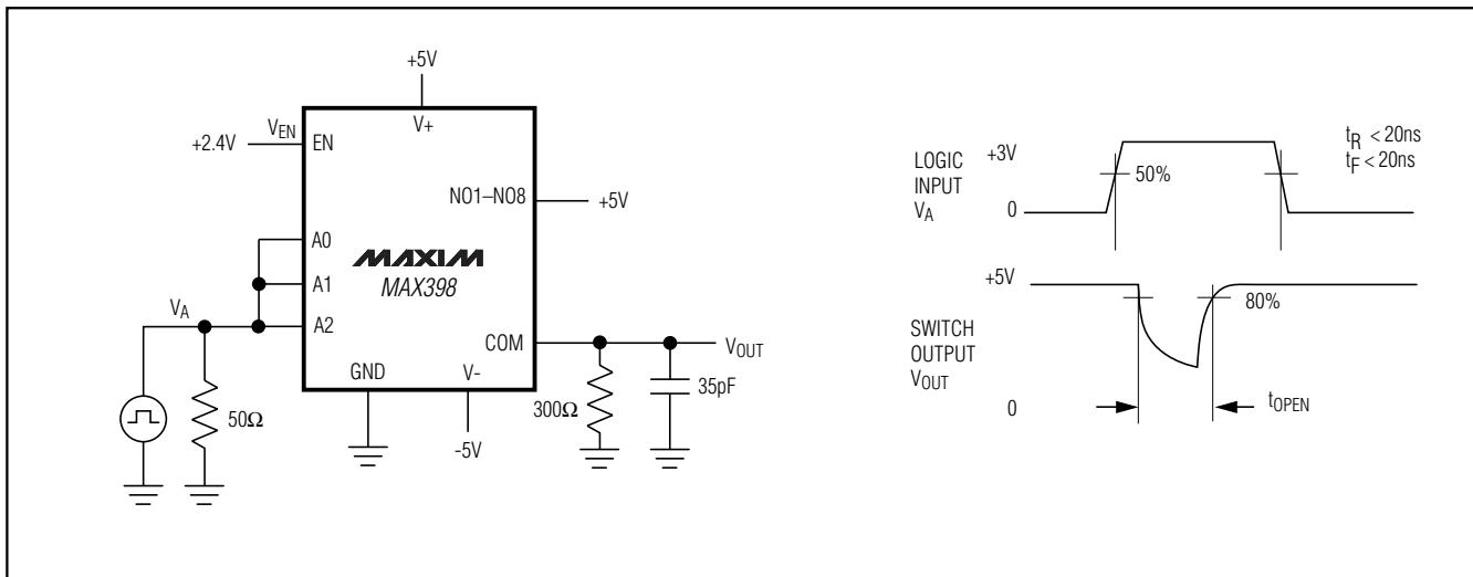
Figure 4. Break-Before-Make Interval
