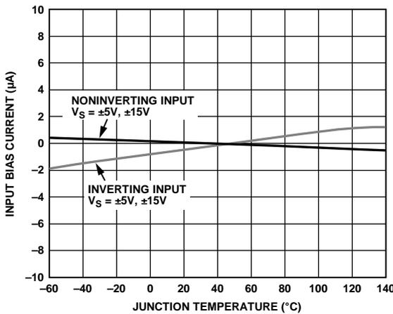
Figure 8. Input Bias Current vs. Junction Temperature
