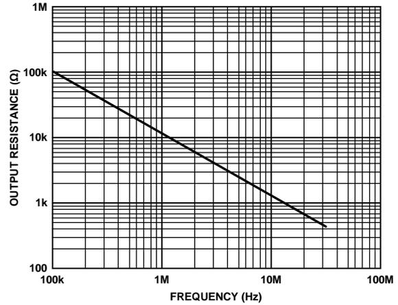
Figure 15. Output Resistance vs. Frequency, Disabled State
