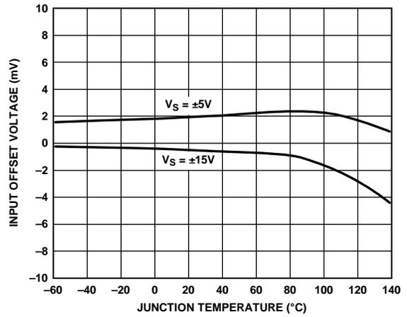
Figure 10. Input Offset Voltage vs. Junction Temperature
