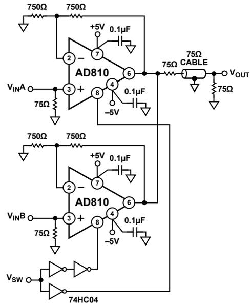
Figure 59. A Fast Switching 2:1 Video Mux
