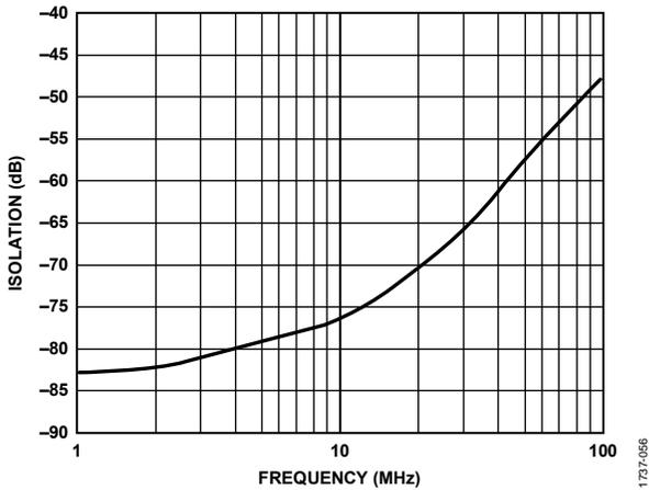
Figure 58. Isolation vs. Frequency for 2:1 Mux, Off Channel
