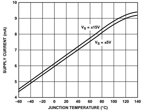
Figure 9. Supply Current vs. Junction Temperature
