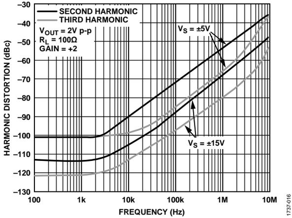
Figure 18. Harmonic Distortion vs. Frequency ( $R_L = 100\ \Omega$ )
