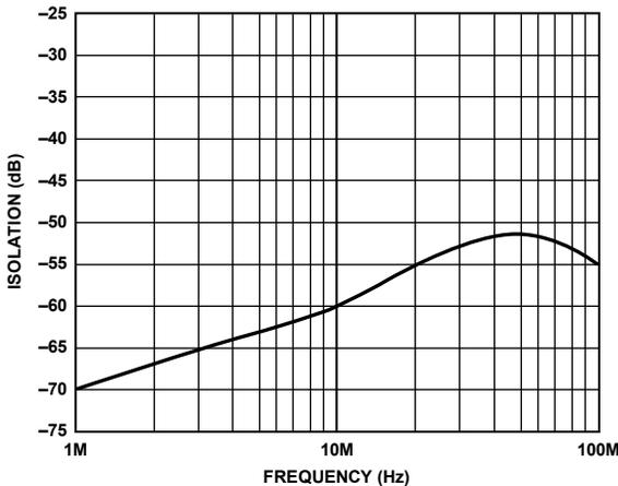
Figure 62. Isolation vs. Frequency for 4:1 Mux, Off Channel
