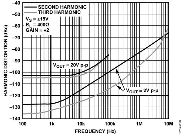
Figure 21. Harmonic Distortion vs. Frequency ( $R_L = 400\ \Omega$ )
