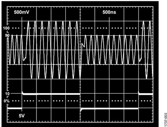
Figure 57. Channel Switching Time for the 2:1 Mux
