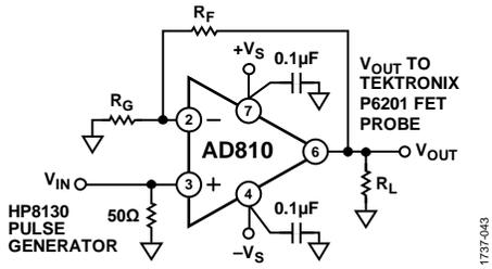
Figure 45. Noninverting Amplifier Connection
