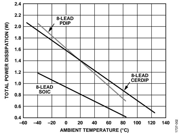
Figure 2. Total Power Dissipation vs. Ambient Temperature
