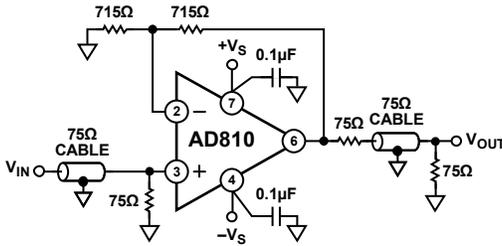
Figure 52. Video Line Driver Operating at Gain = +2
