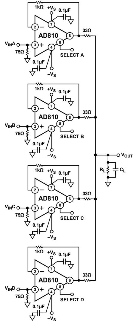
Figure 63. 4:1 Multiplexer Driving a High Impedance
