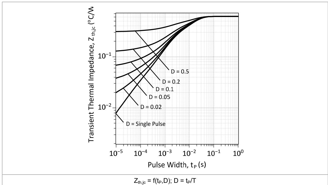
**Figure 9: Transient Thermal Impedance**
