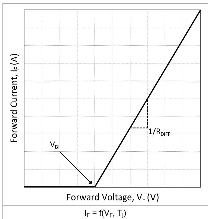
$$I_F = (V_F - V_{BI})/R_{DIFF} \text{ (A)}$$
