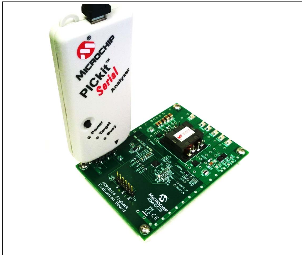
FIGURE 3-1: PICKit Serial Analyzer Connection to the Board.
