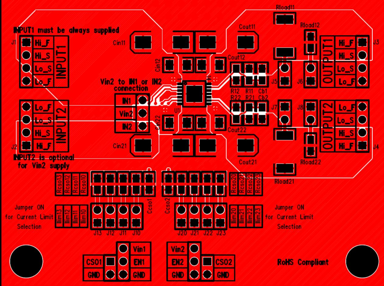
Figure 2. Top side PCB Layout (3 x 3 inch)
