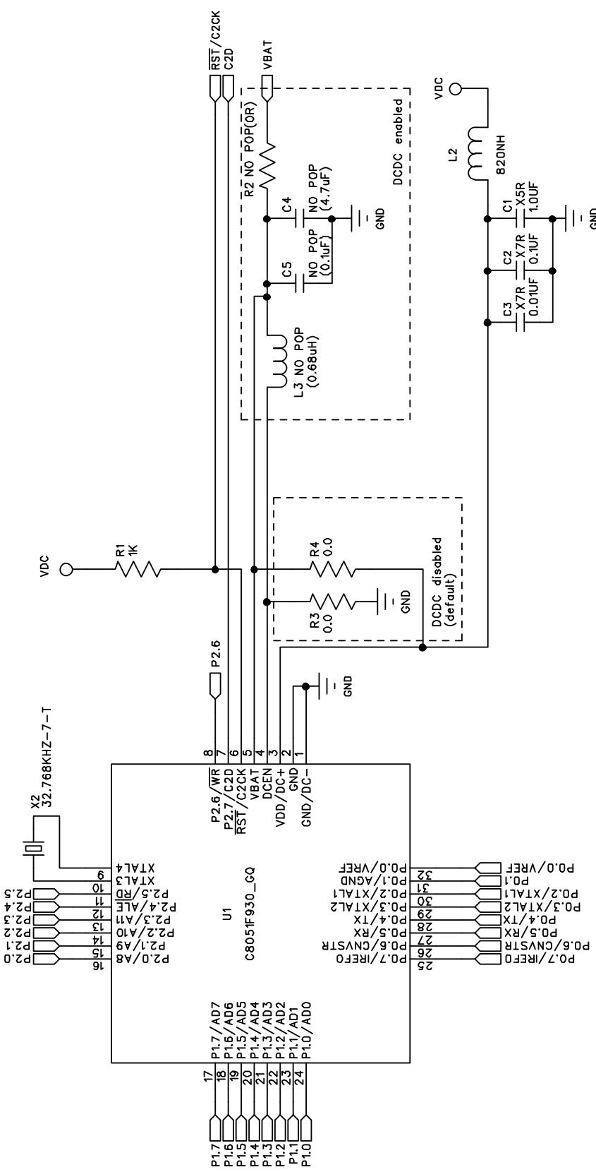
Figure 11. UPPI-930-RF MCU Pico Board Schematic (1 of 2)
