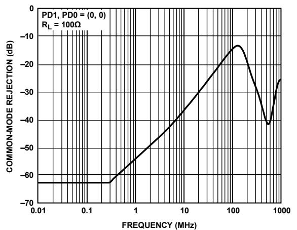
Figure 13. Common-Mode Rejection(CMR) vs. Frequency
