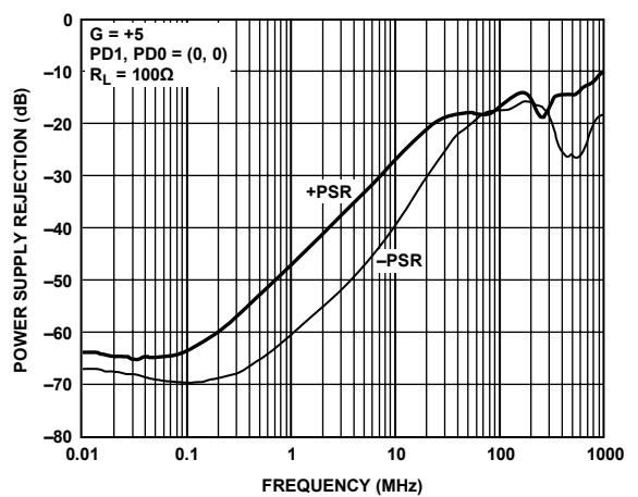
Figure 14. Power Supply Rejection(PSR) vs. Frequency
