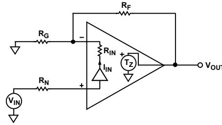
Figure 20. Simplified Block Diagram
