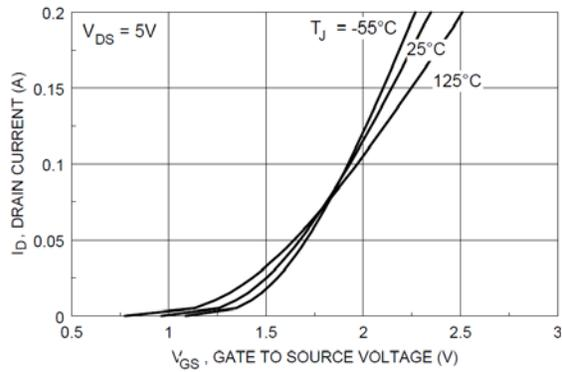
Figure 5. Transfer Characteristics.
