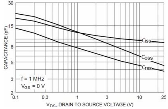
Figure 8. Capacitance Characteristics.
