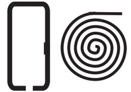
Figure 127: Loop or Trace Antenna
