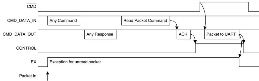
Figure 22: HumPRO™ Series Transceiver Received Packet Transfer Cycle
