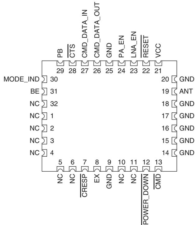
Figure 14: HumPRO™ Series Transceiver Pin Assignments (Top View)
