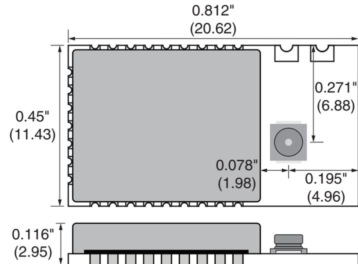
Figure 19: HumPRO™ Series Transceiver Pre-certified Version Dimensions
