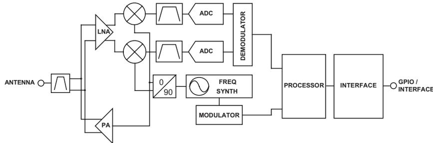
Figure 20: HumPRO™ Series Transceiver RF Section Block Diagram
