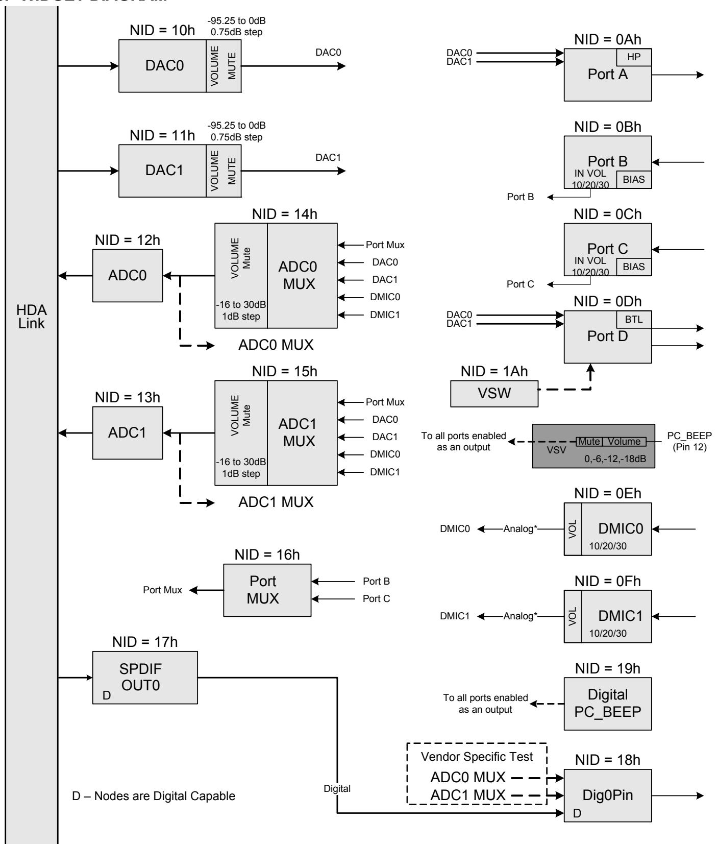
Figure 13. Widget Diagram
