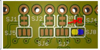
To free up Arduino **pin 8**, the Mux Shield must use all 48 I/O's as either all inputs (analog or digital) or all outputs. This is because pin 8 is used as a control signal gate and chip enable signal. If pin 8 is freed up, pins 10, 11, and 12 are no longer needed and can be disconnected using the directions above.
