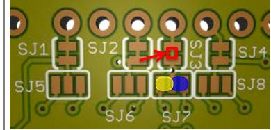
To free up Arduino pin 12, and hardwire row I/O3 as either input or output:
