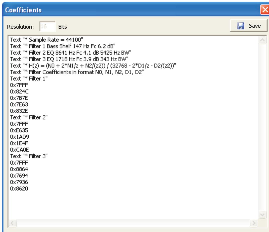
**Figure 6. Filter Coefficients**
