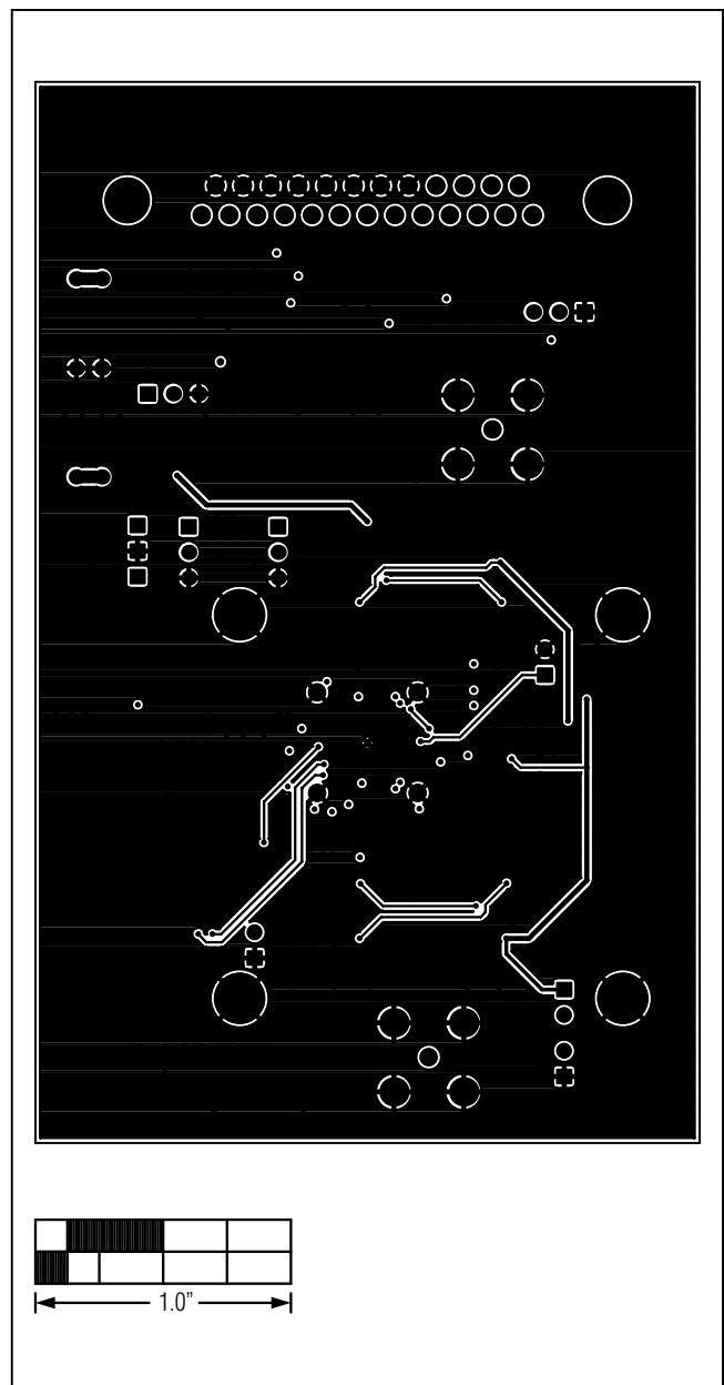
Figure 5. MAX2140 EV Kit PCB Layout—Layer 3
