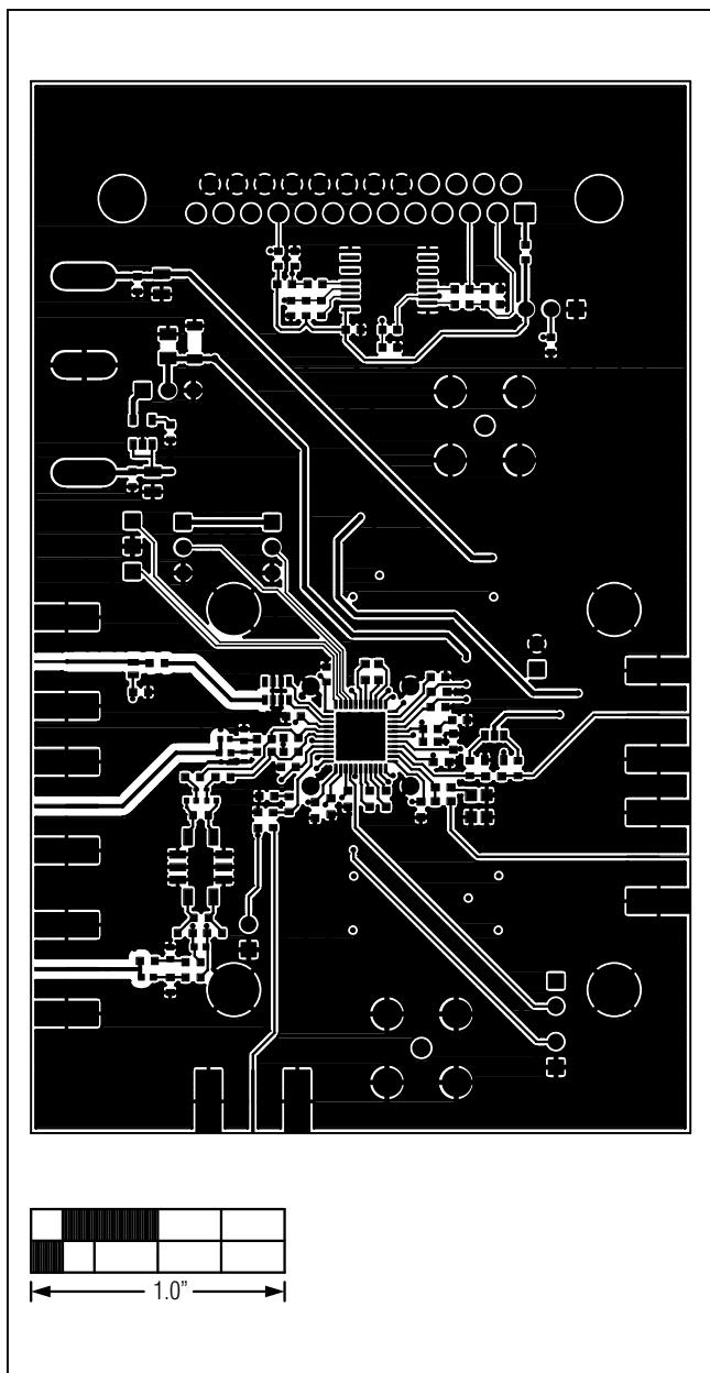
Figure 6. MAX2140 EV Kit PCB Layout—Component Side
