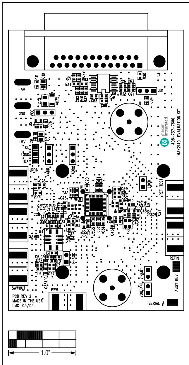
Figure 2. MAX2140 EV Kit Component Placement Guide—
