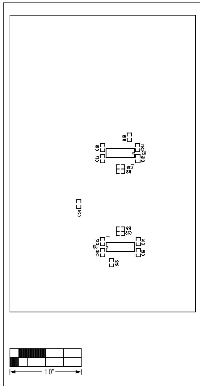
Figure 3. MAX2140 EV Kit Component Placement Guide—
