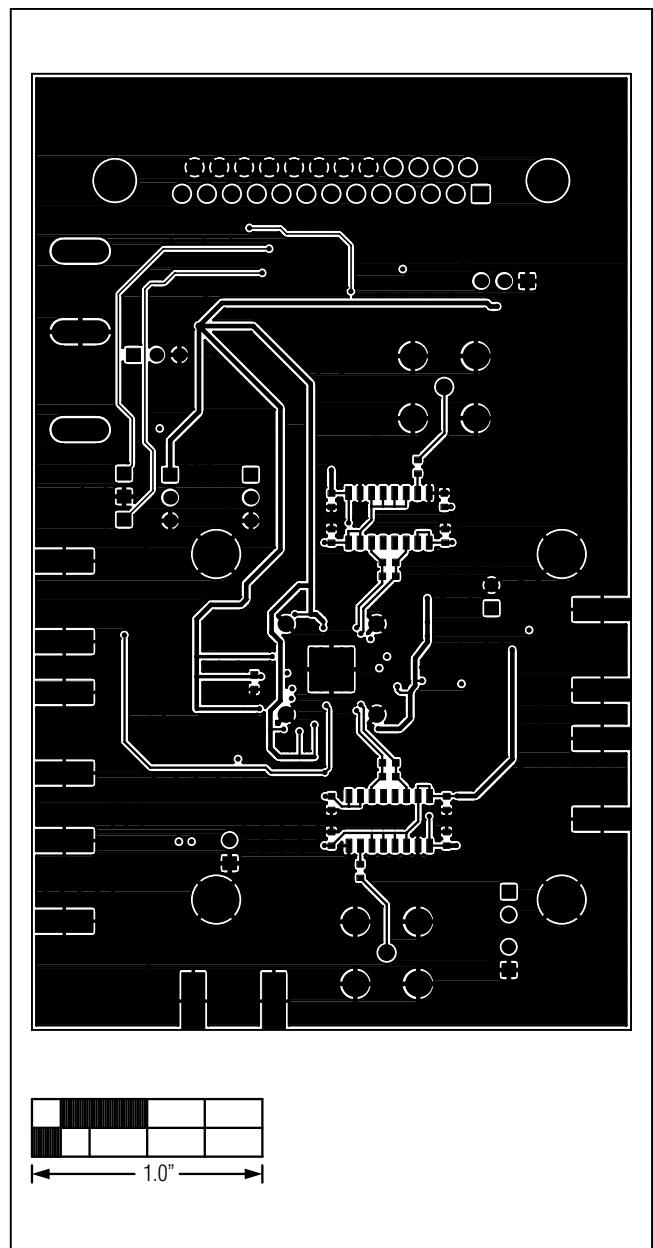
Figure 7. MAX2140 EV Kit PCB Layout—Secondary Side
