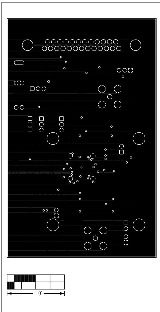
Figure 4. MAX2140 EV Kit PCB Layout—Layer 2
