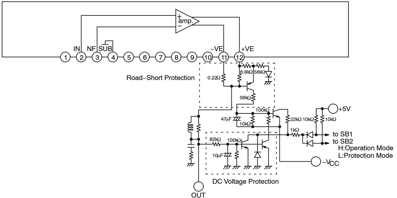
Figure 29. STK404-120N-E Road-short & DC Voltage Protection Application
