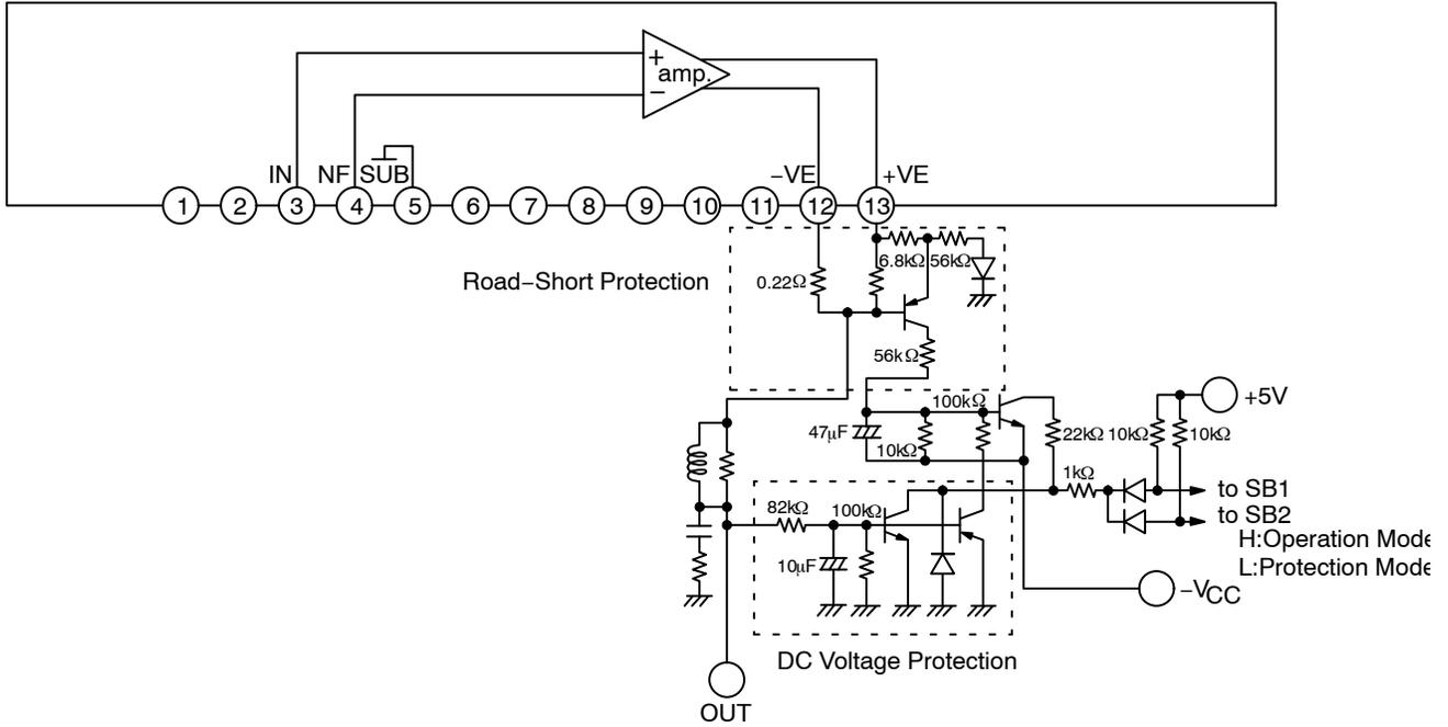
Figure 30. STK404-140N-E Road-short & DC Voltage Protection Application
