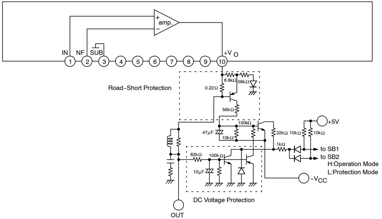
Figure 28. STK404-070N-E Road-short & DC Voltage Protection Application
