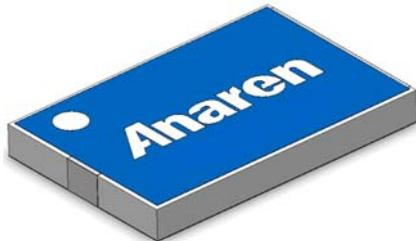
The C200N50Z4 is high performance Aluminum Nitride (AlN) surface mount termination intended as a cost competitive alternative to Beryllium Oxide (BeO). The termination is well suited to all cellular frequency bands such as; AMPS, GSM, DCS, PCS, PHS and UMTS. The high power handling makes the part ideal for terminating high power 90 degree couplers and for use in microstrip circuits. The termination is also RoHS compliant!
