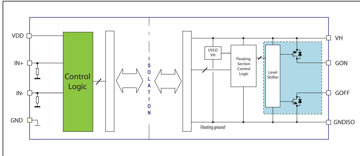
**Figure 2. Block diagram - single output and Miller clamp option**
