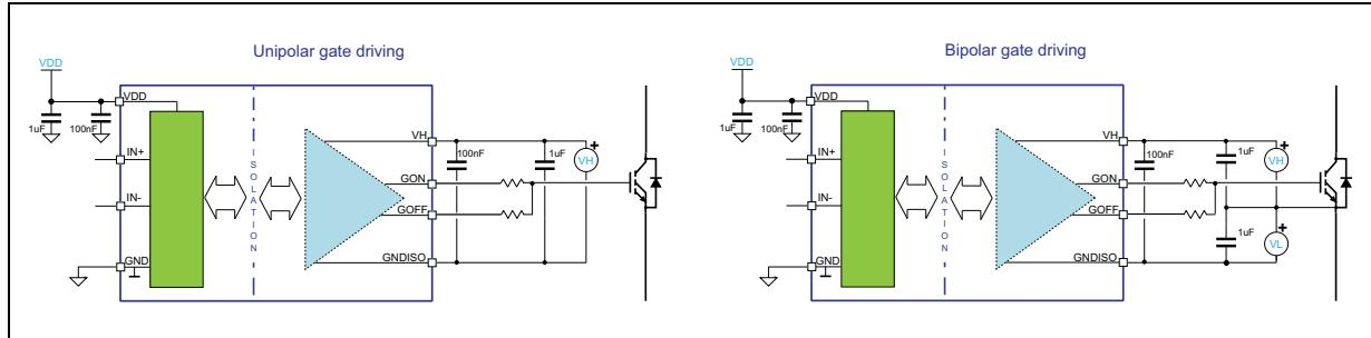
Undervoltage protection is available on VH supply pin. A fixed hysteresis sets the turn-off threshold, thus avoiding intermittent operation.
