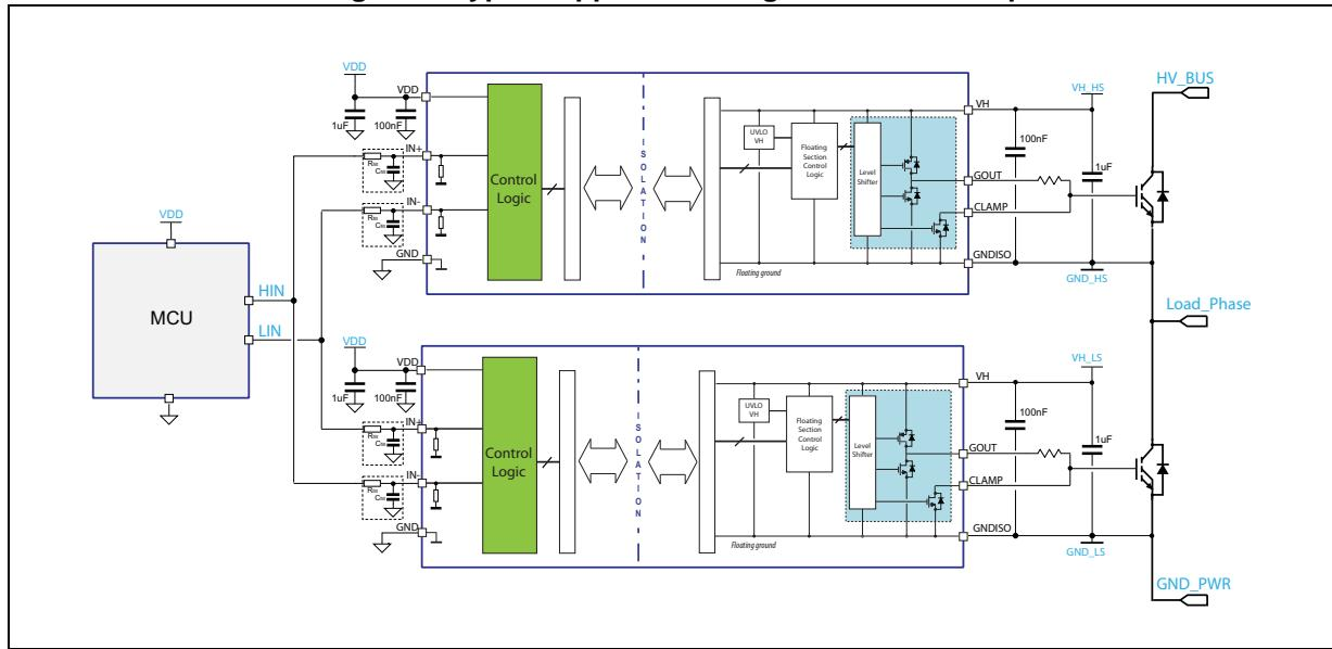
**Figure 10. Typical application diagram - Miller clamp and negative gate driving**
