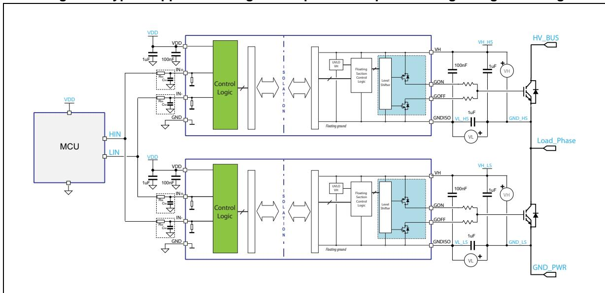
**Figure 9. Typical application diagram - Miller clamp**
