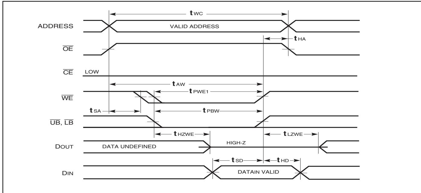
**WRITE CYCLE NO. 3** ( $\overline{WE}$  Controlled.  $\overline{OE}$  is LOW During Write Cycle) <sup>(1)</sup>
