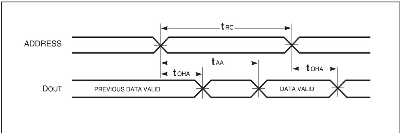
**READ CYCLE NO. 2<sup>(1,3)</sup>** ( $\overline{CE}$  and  $\overline{OE}$  Controlled)
