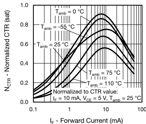
Fig. 12 - Normalized CTR (saturated) vs. Forward Current
