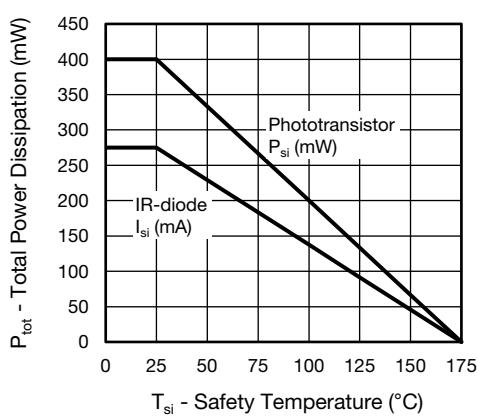
Fig. 1 - Total Power Dissipation vs. Safety Temperature
