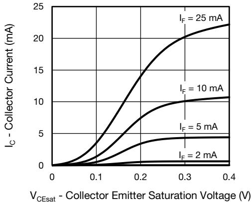
Fig. 8 - Collector Current vs. Collector Emitter Voltage (saturated)
