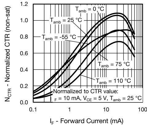
Fig. 11 - Normalized CTR (non-saturated) vs. Forward Current
