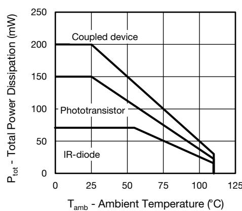
Fig. 2 - Total Power Dissipation vs. Ambient Temperature
