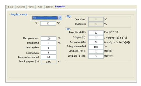
The picture shows the function of the PID regulator.
