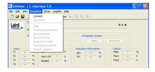
**Connect** To connect regulator board to serial interface connection.
