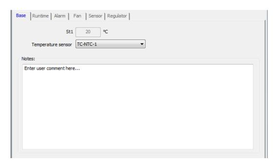
Base tab allows for quick setup of the regulator. Select temperature sensor, set point and enter description information under notes to recall settings for future reference. All data will be stored in the file.
