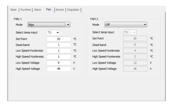
The FAN tab allows user to control two fans (hot side fan and cold side fan) independently by turning on fans permanently, only in heating mode and/or cooling mode, during specific temperature set points, during specific hysteresis range, under specified voltage limits or turning off during specific dead bands.
