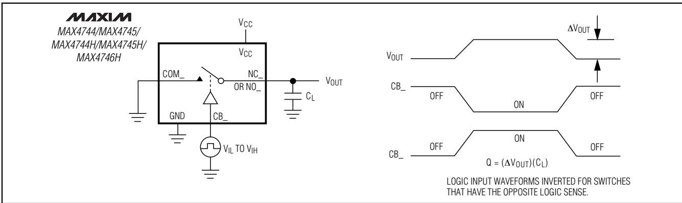
Figure 4. Charge Injection
