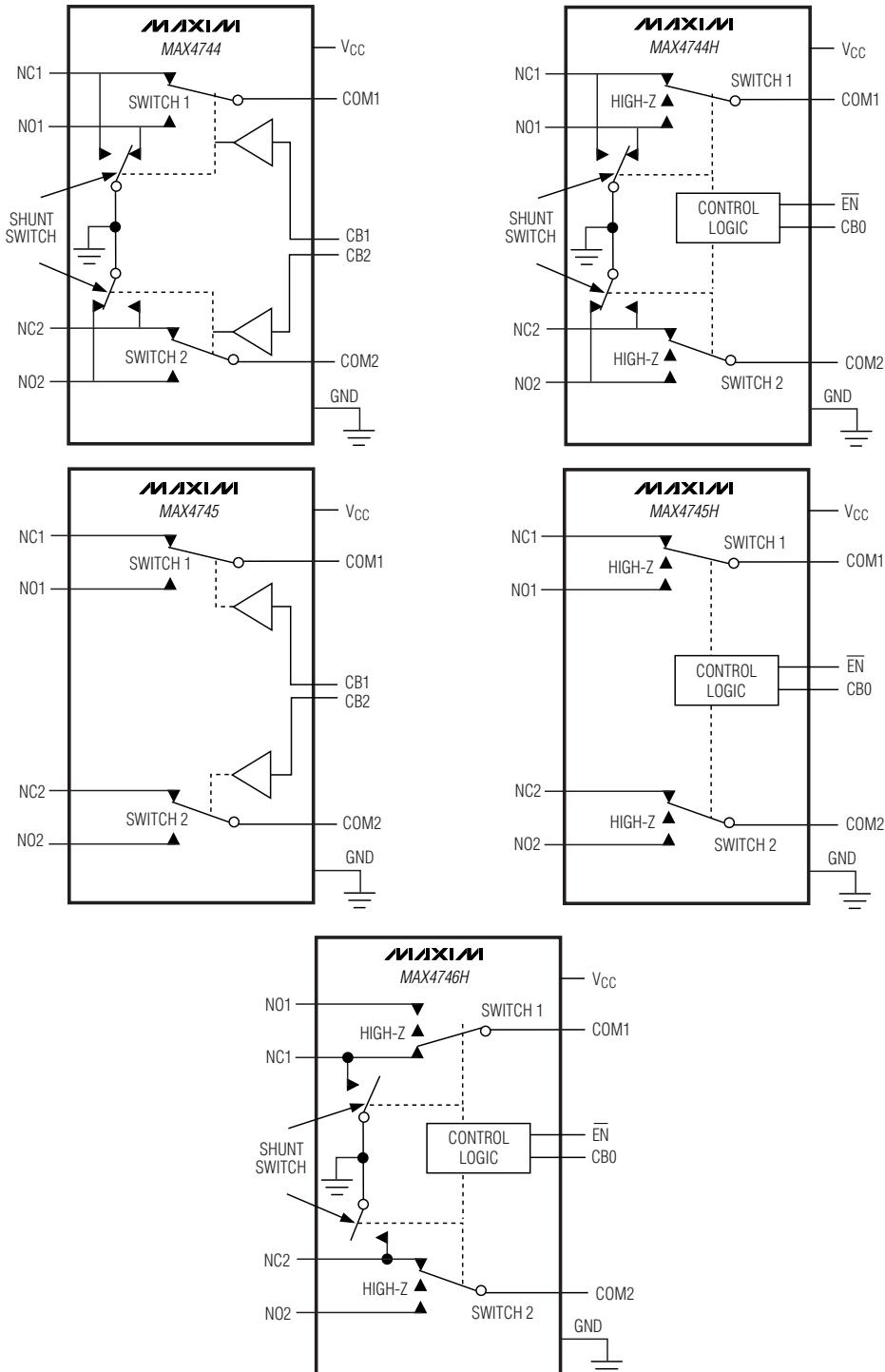
Figure 1. Functional Diagram
