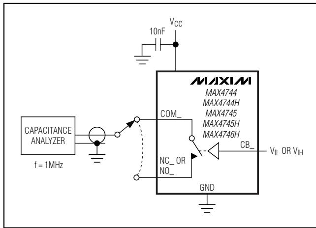
Figure 6. Channel Off-/On-Capacitance
