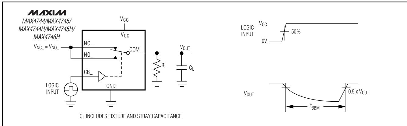
Figure 3. Break-Before-Make Interval
