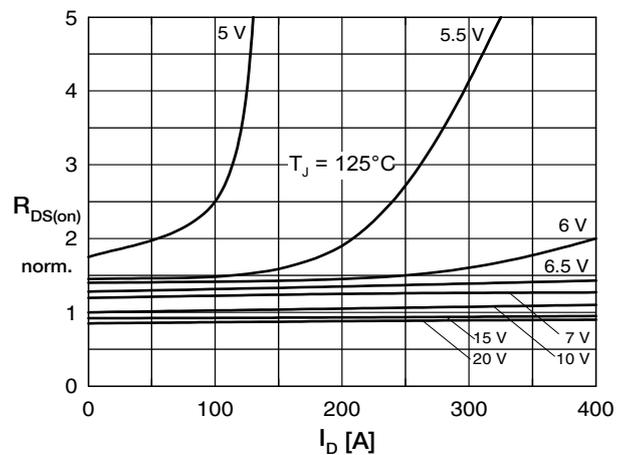
Fig. 6 Drain source on-state resistance  $R_{DS(on)}$  versus  $I_D$ , on die level
