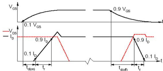
Fig. 17 Definition of switching times
