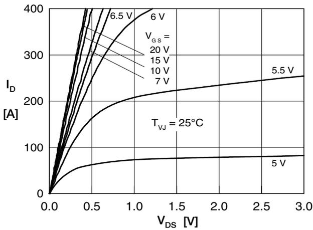
Fig. 3 Typ. output characteristics on die level
