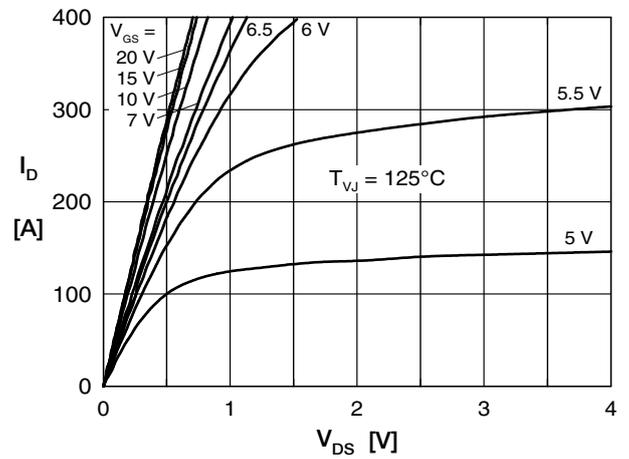
Fig. 4 Typ. output characteristics on die level
