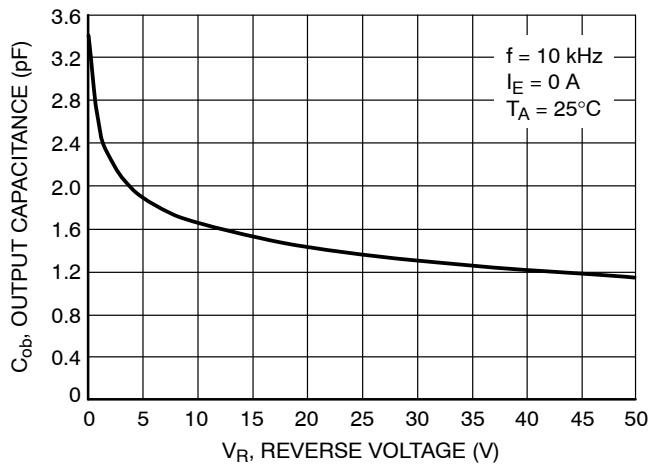
**Figure 4.** Output Capacitance
