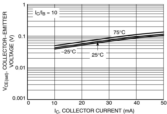
**Figure 2.**  $V_{CE(\text{sat})}$  vs.  $I_C$
