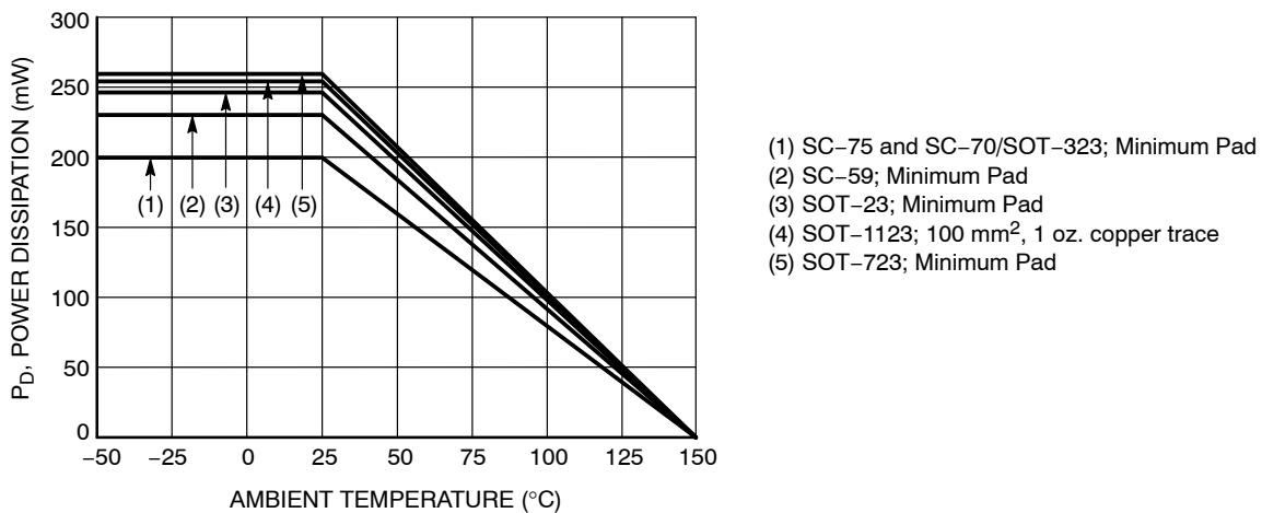
**Figure 1. Derating Curve**
