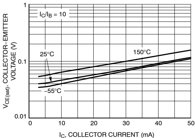
Figure 7.  $V_{CE(\text{sat})}$  vs.  $I_C$
