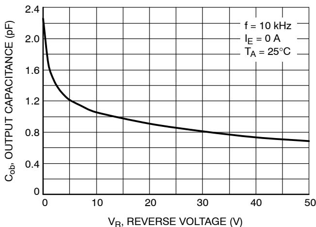
Figure 9. Output Capacitance
