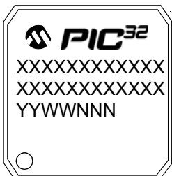
100-Lead TQFP (14x14x1 mm)
