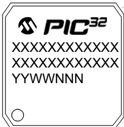
100-Lead TQFP (12x12x1 mm)
