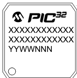
100-Lead TQFP (12x12x1 mm)
