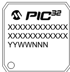
100-Lead TQFP (14x14x1 mm)
