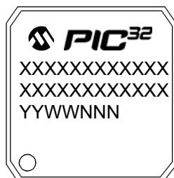
100-Lead TQFP (12x12x1 mm)
