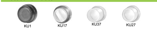
These 9001KU protective boots are recommended for very dirty environments or severe hose down, but they are not required for UL Type 4 or 4X rating on the 9001SK operators. The 9001K1 wrench (see page 59) is required for installation of these boots.
