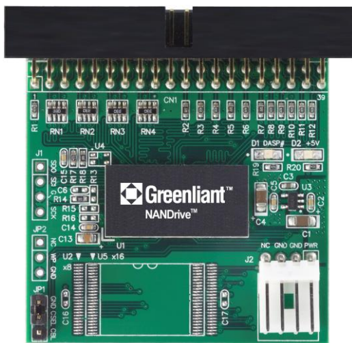
Figure 1: NANDrive Evaluation Board, 40-pin Connector
