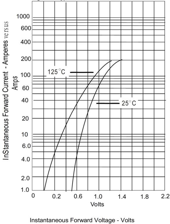
Figure .2- Forward Derating Curve
