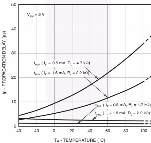
**Fig. 14 Propagation Delay vs. Temperature
