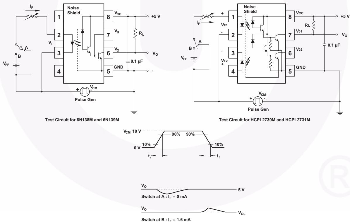
Fig. 16 Common Mode Immunity Test Circuit
