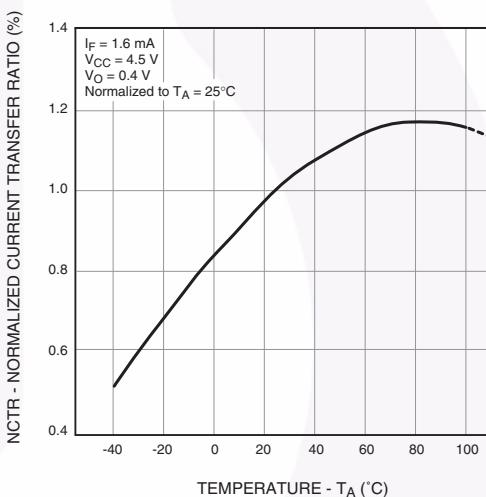
Fig. 9 Normalized Current Transfer Ratio
