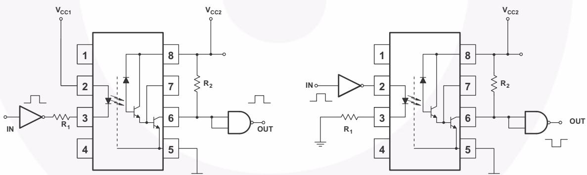
Fig. 4 Non-Inverting Logic Interface
