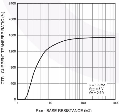
Fig. 10 Current Transfer Ratio vs. Base-Emitter Resistance
