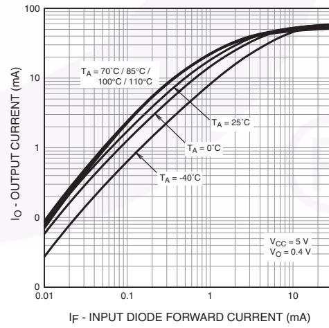
Fig. 11 Output Current vs. Input Diode Forward Current
