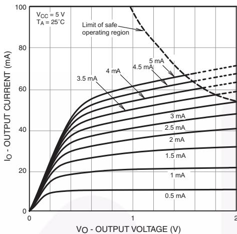
**Fig. 12 Output Current vs Output Voltage
