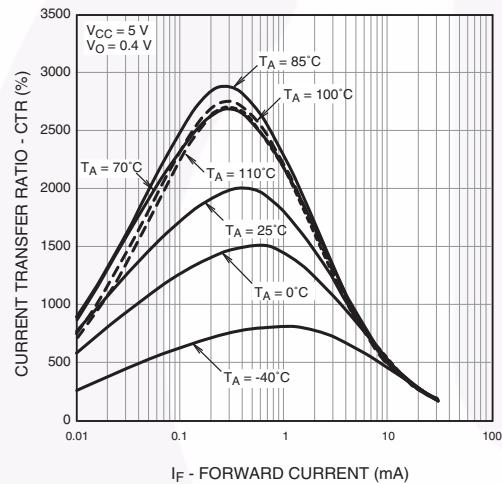
Fig. 8 Current Transfer Ratio vs. Forward Current
