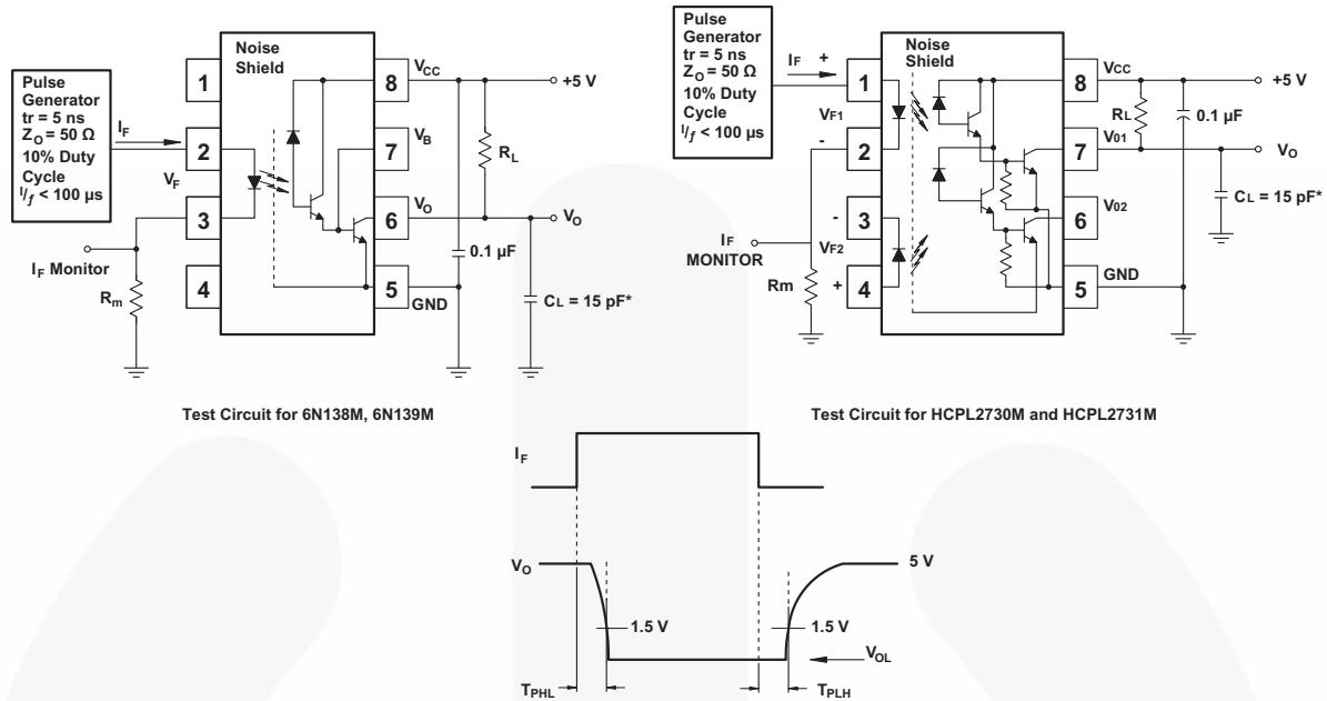
Fig. 15 Switching Time Test Circuit
