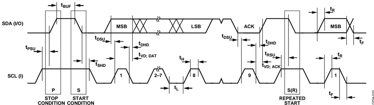
Figure 2. I<sup>2</sup>C Compatible Interface Timing
