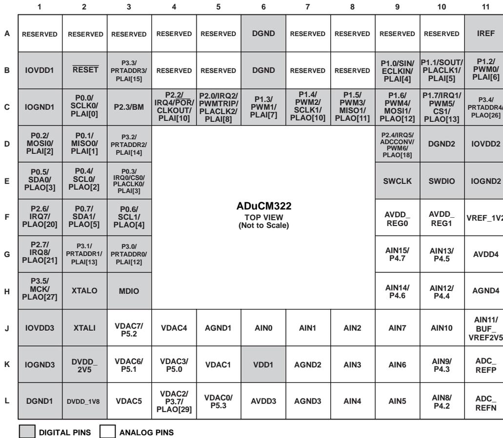
Figure 8. Pin Configuration
