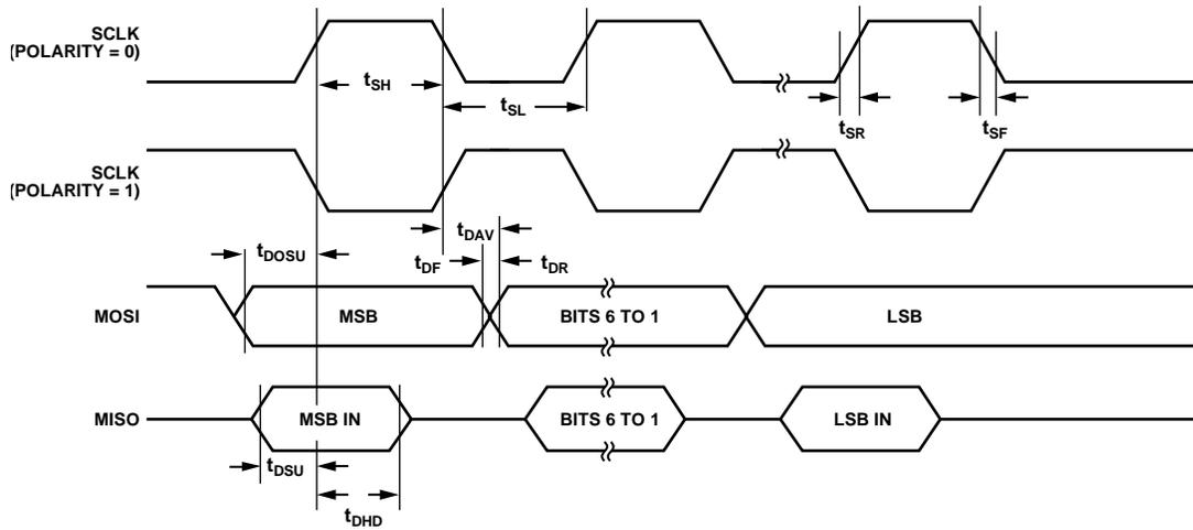
Figure 4. SPI Master Mode Timing (Phase Mode = 0)
