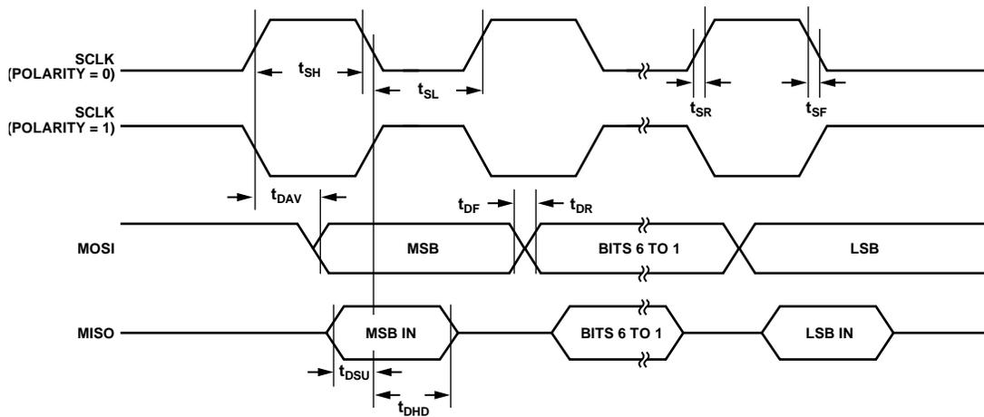
Figure 3. SPI Master Mode Timing (Phase Mode = 1)
