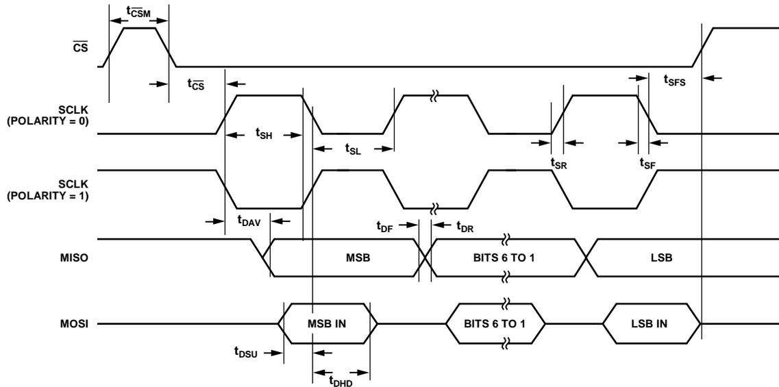
Figure 5. SPI Slave Mode Timing (Phase Mode = 1)
