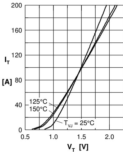
Fig. 1 Forward characteristics
