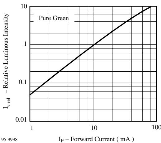
Figure 18 Relative Luminous Intensity vs.
