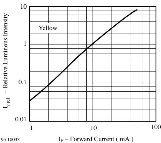
Figure 8 Relative Luminous Intensity vs. Forward Current
