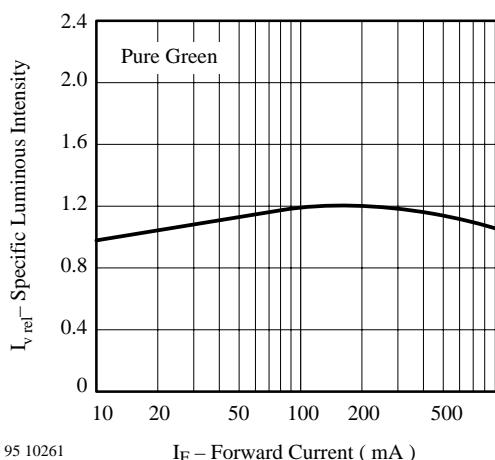
Figure 17 Specific Luminous Intensity vs.
