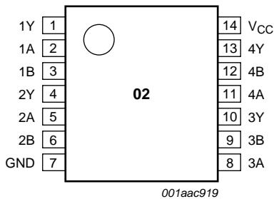
Fig 4. Pin configuration SO14 and (T)SSOP14
