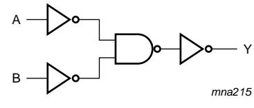
Fig 3. Logic diagram for one gate
