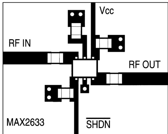
Figure 7. MAX2633 Example PC Board Layout
