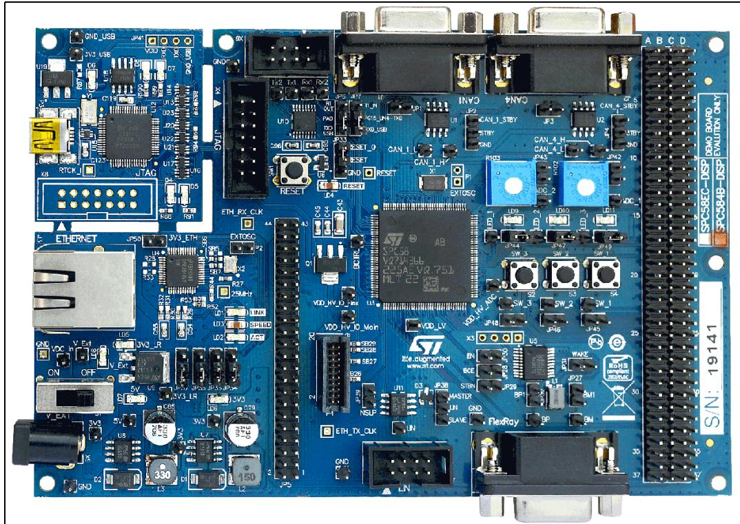
The several interfaces including Ethernet controller, CAN-FD, FlexRay, LIN and UART, ADC, and JTAG port make the SPC584B-DISP an excellent tool to evaluate the microcontroller as well as to develop and then debug applications.
