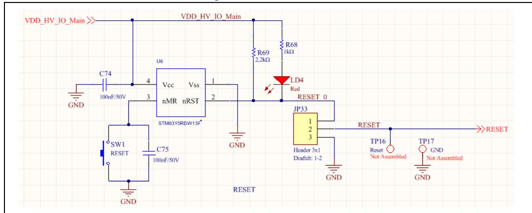
The device generates a reset signal when the SW1 button is pressed.
