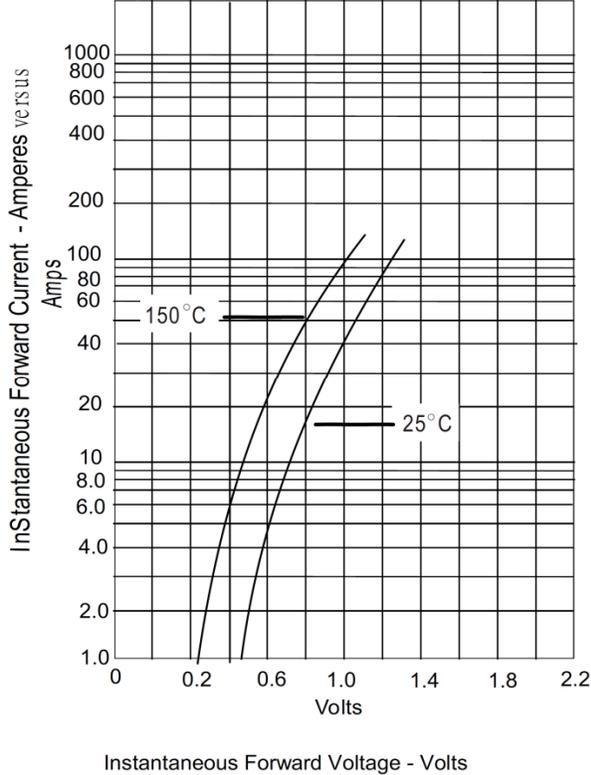
Figure .2-Forward Derating Curve
