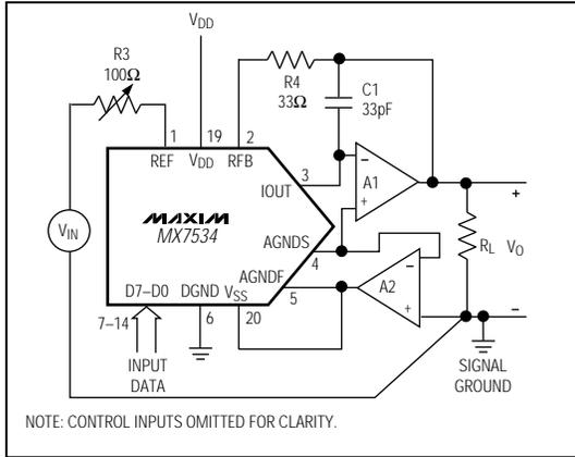
Figure 6a. Unipolar Binary Operation with Forced Ground
