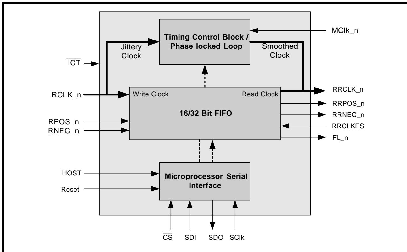
The XRT71D03 DS3/E3 Jitter Attenuator IC consists of the following functional blocks:
