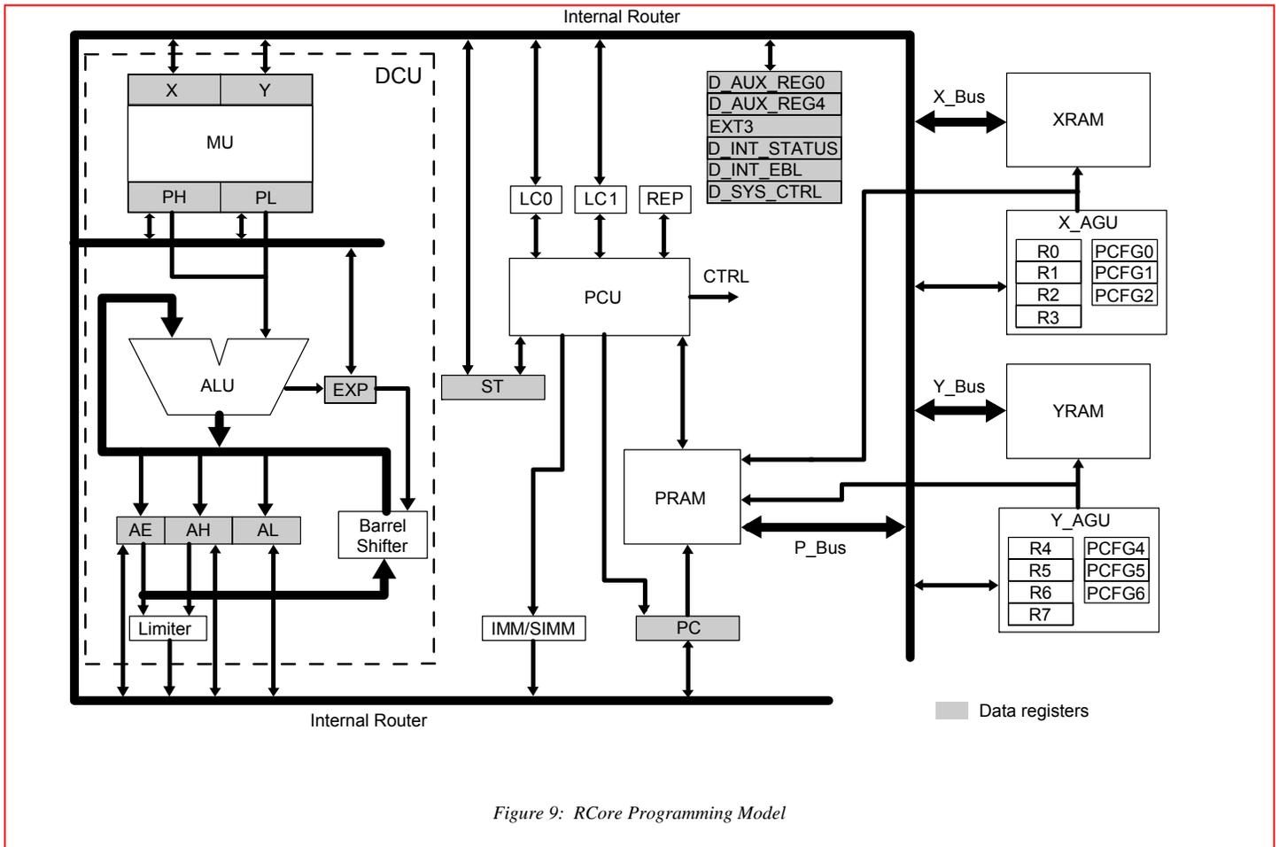
Figure 9: RCore Programming Model
