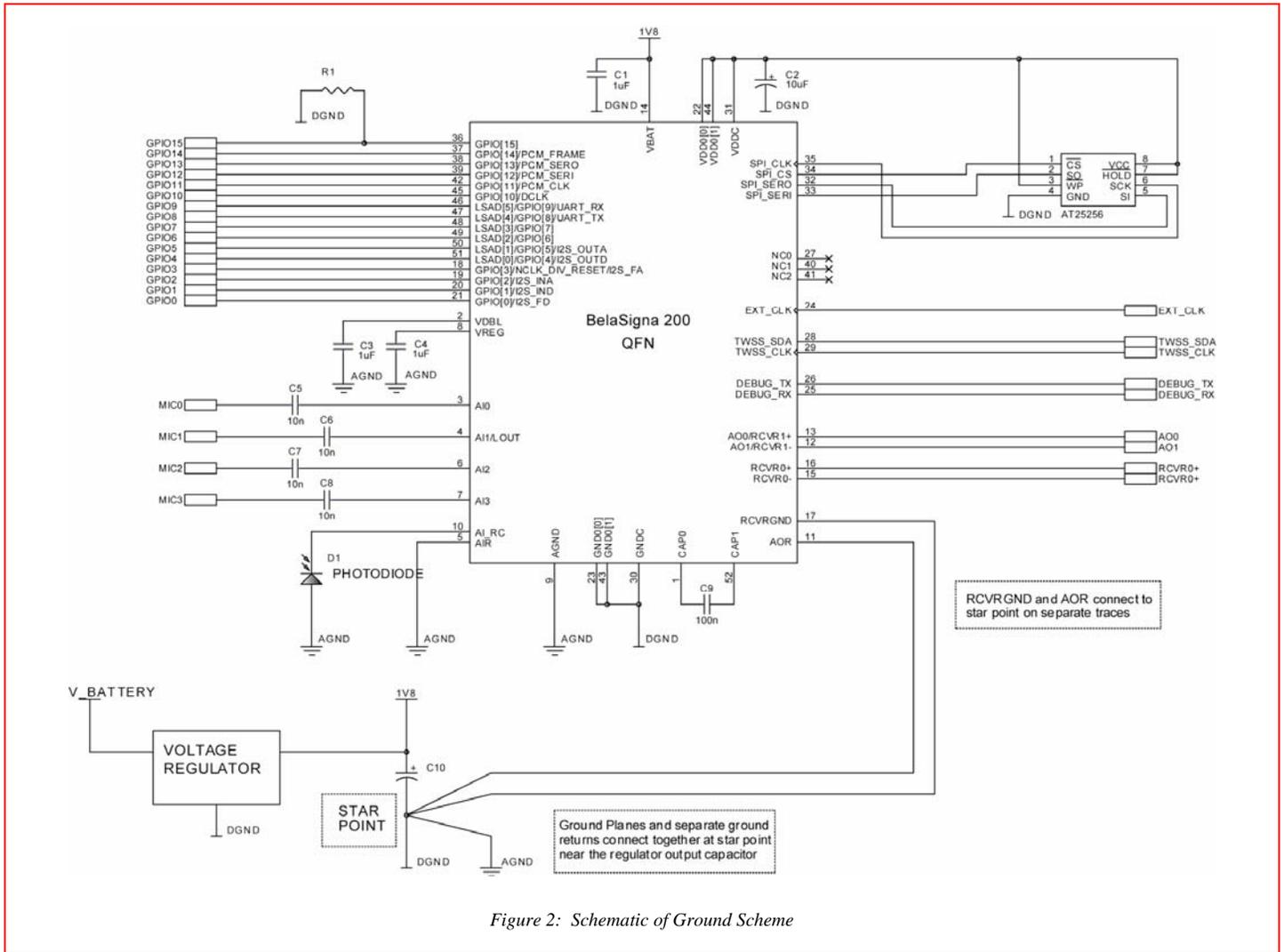
Figure 2: Schematic of Ground Scheme
