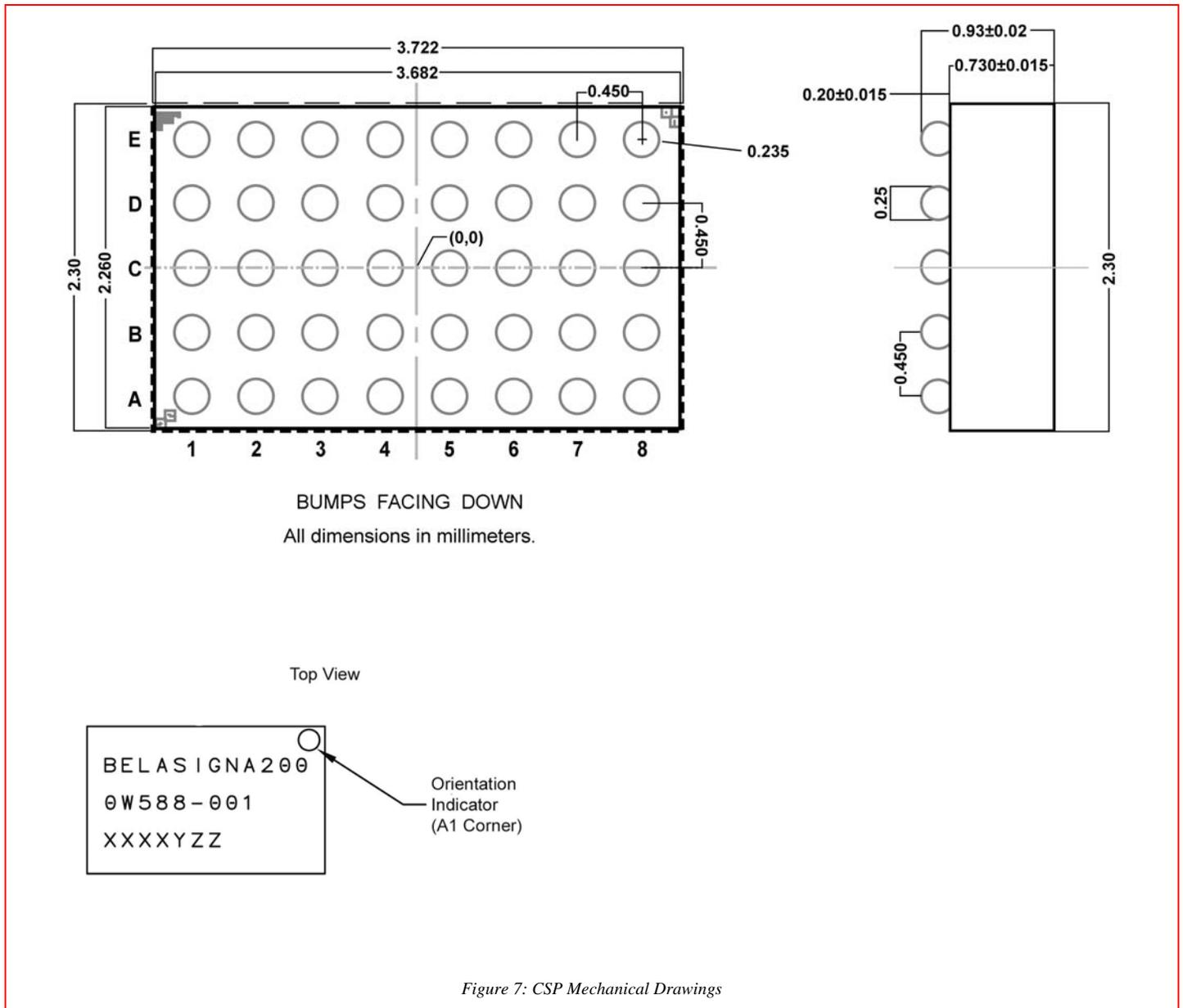
Figure 7: CSP Mechanical Drawings
