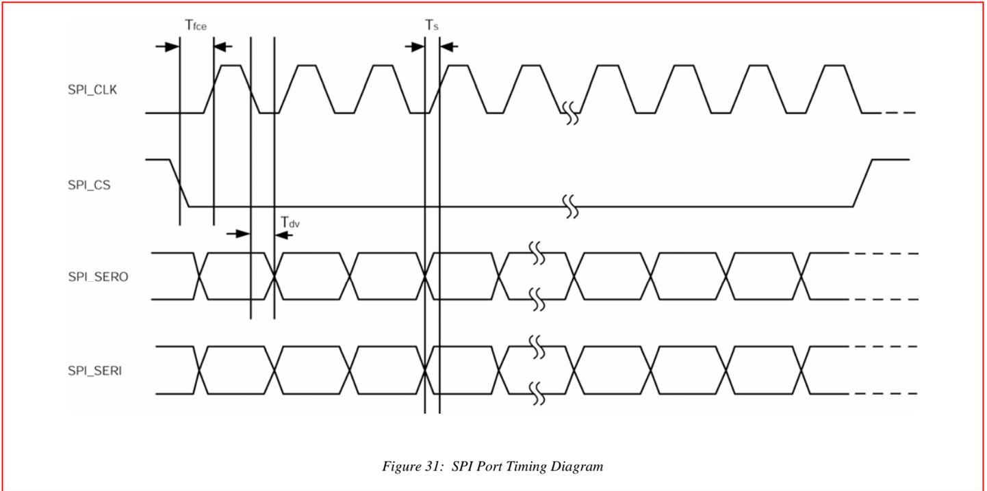
Figure 31: SPI Port Timing Diagram
