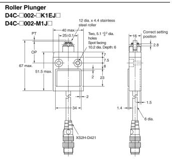
Note: Unless otherwise specified, a tolerance of  $\pm 0.4 \ \text{mm}$  applies to all dimensions.
