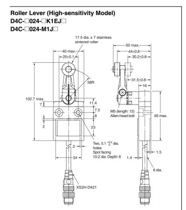
Note: Unless otherwise specified, a tolerance of  $\pm 0.4 \ \text{mm}$  applies to all dimensions.
