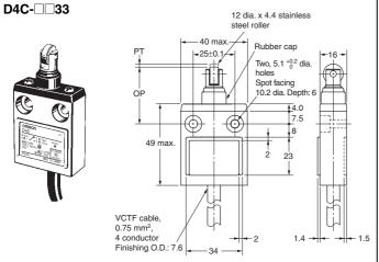
Note: Unless otherwise specified, a tolerance of  $\pm 0.4$  mm applies to all dimensions.
