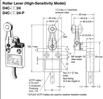
Note: Unless otherwise specified, a tolerance of  $\pm 0.4 \ \text{mm}$  applies to all dimensions.
