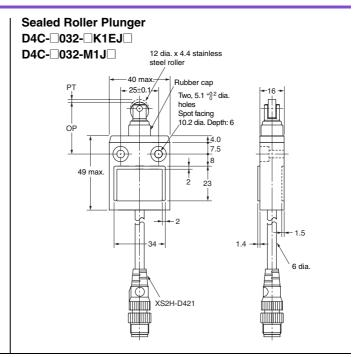
Note: Unless otherwise specified, a tolerance of  $\pm 0.4$  mm applies to all dimensions.
