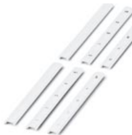
Zack Marker strip, flat, Strip, white, Unlabeled, Can be labeled with: Plotter, Mounting type: Snap into flat marker groove, Lettering field: 15 x 5.2 mm
