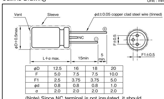
(Note) Since NC terminal is not insulated, it should be mounted at a position electronically independent from all other parts of the circuit.
