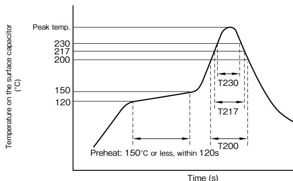
T200 : Duration while capacitor head temperature exceeds 200°C (s)
