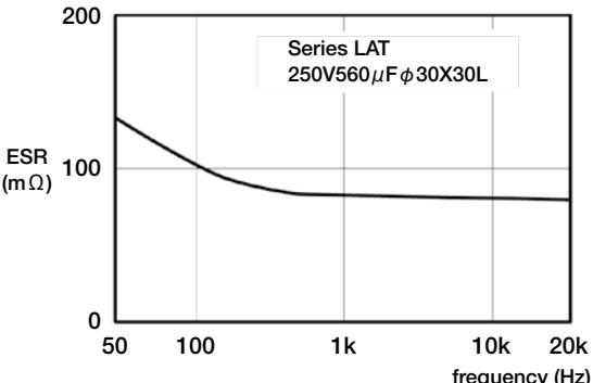
Figure 2-5 shows a typical example of frequency characteristics of ESR, indicating that the ESR decreases with increasing frequencies. Therefore, the high-frequency component has less effect on the heat generation of capacitor than low-frequency component.
