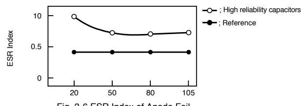
Fig. 3-6 ESR Index of Anode Foil
