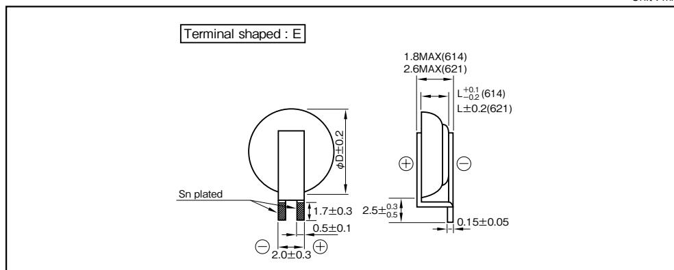
Part numbering system (example : 614,2.5V0.2F, terminal shaped : E)
